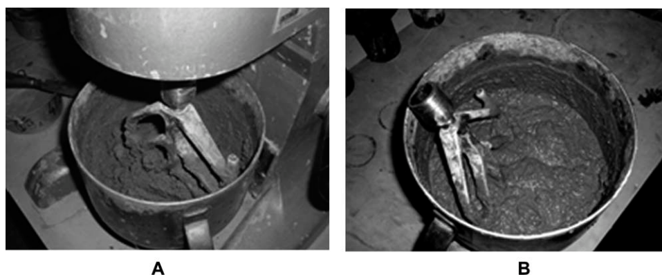
Figure 4 (A) Mortar without polymer (reference) and (B) mortar containing polymer (NMC).
